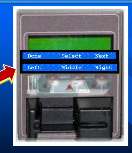
To access the CAD Diagnostic Screen, press the left button for @ least 3 seconds
